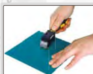
step 1: make grid cutting on surface
