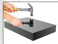
hammer impact to apply test force
