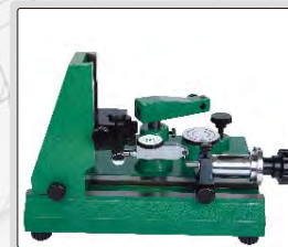
inspect accuracy of test indicators
