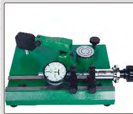
inspect accuracy of dial indicators (range 0-25mm)
