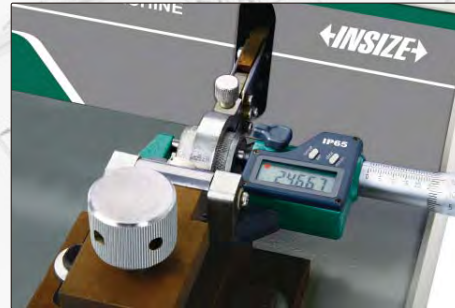
lapping measuring surfaces of outside micrometer
