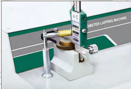
lapping measuring surfaces of caliper lower jaws
