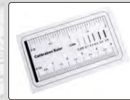
plastic calibration rule (included, graduation 1mm)
