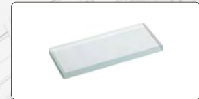
50mm reading scale (check magnification accuracy)
