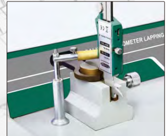
lapping measuring surfaces of caliper lower jaws
