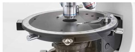
Center-adjustable and turnable polarisation stage
