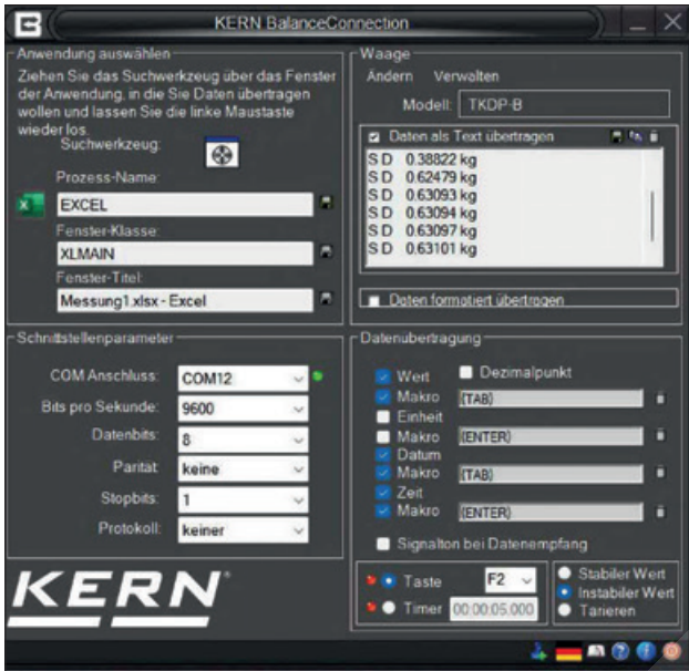
Programme start and quick configuration of the RS232/USB interface
