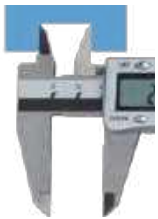
Innenmessung / internal measuring
