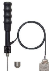
HH-V400 impact device HLDL scale Use for gear teeth, welded corners, etc.
