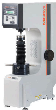
HR-430MR Rockwell hardness testing machine:
