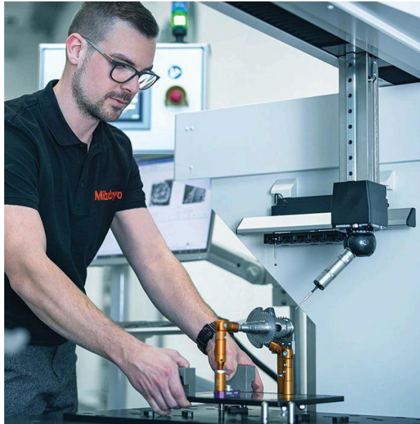
3-point repositioning Pallet Receiver System PRS
