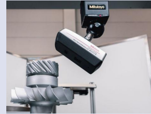
The flying spot type is capable of scanning difficult parts, such as this impeller, precisely and achieves highest scanning accuracy in the class.
