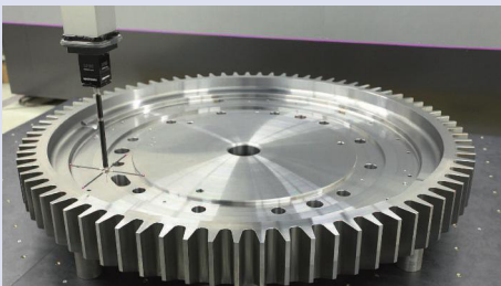
Scanning with probe SP80 and 100 mm styli.
