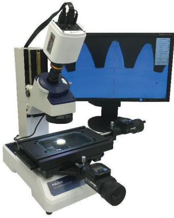
TM-1005B with 2x digimatic micrometer heads and 63AAA353 camera set
