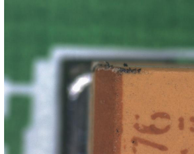
Normal microscope observation (upper) With a height difference, only the upper or lower plane can be focused.
