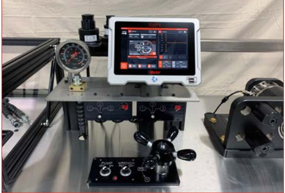
T-Box™ 2 at the center of a test bench for manual torque wrenches, powered torque tools and hydraulic torque wrenches
