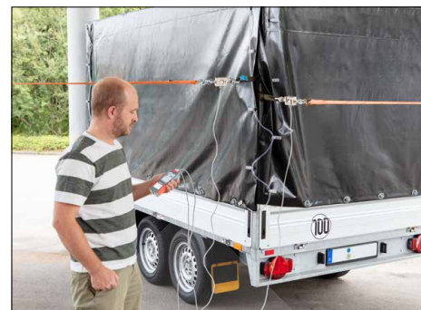
Measurement of forces in different tensile or compression directions possible with only one measuring device
