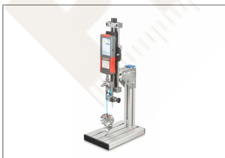
Can be mounted on all SAUTER test stands, illustration shows optional accessories, as well as the SAUTER TVL-XS manual test stand
