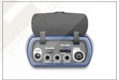
...and data transfer using MicroSD (4G) memory card (included in delivery), RS-232 or USB
