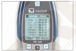
Data logging function with date and time in the device....
